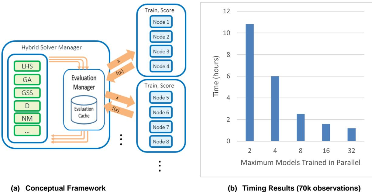
Figure 10. Distributed/Parallel Training and Parallel Tuning Combined
