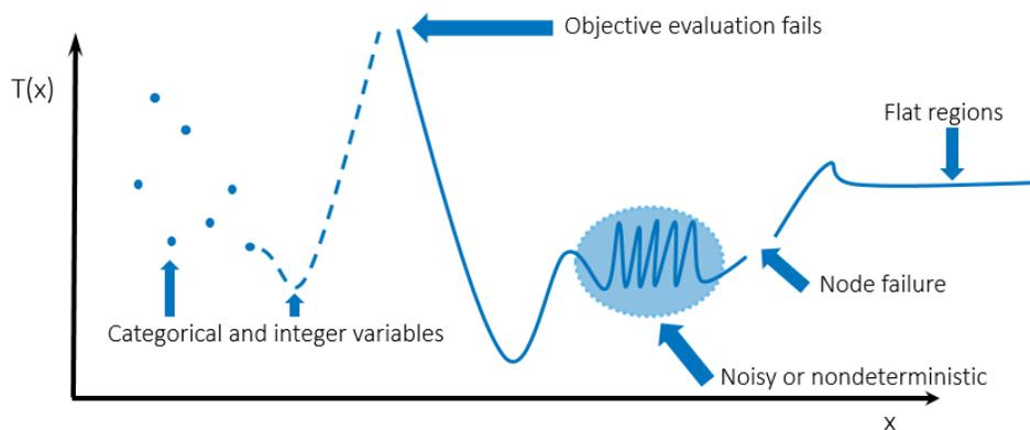
**Figure 5. Challenges in Applying Optimization to Hyperparameter Tuning**
